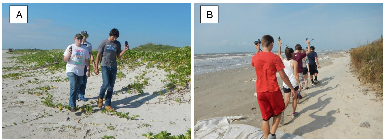
Figure 5-3. Students mapping (A) the vegetation line and (B) shoreline (wet/dry line) using handheld GPS units.
