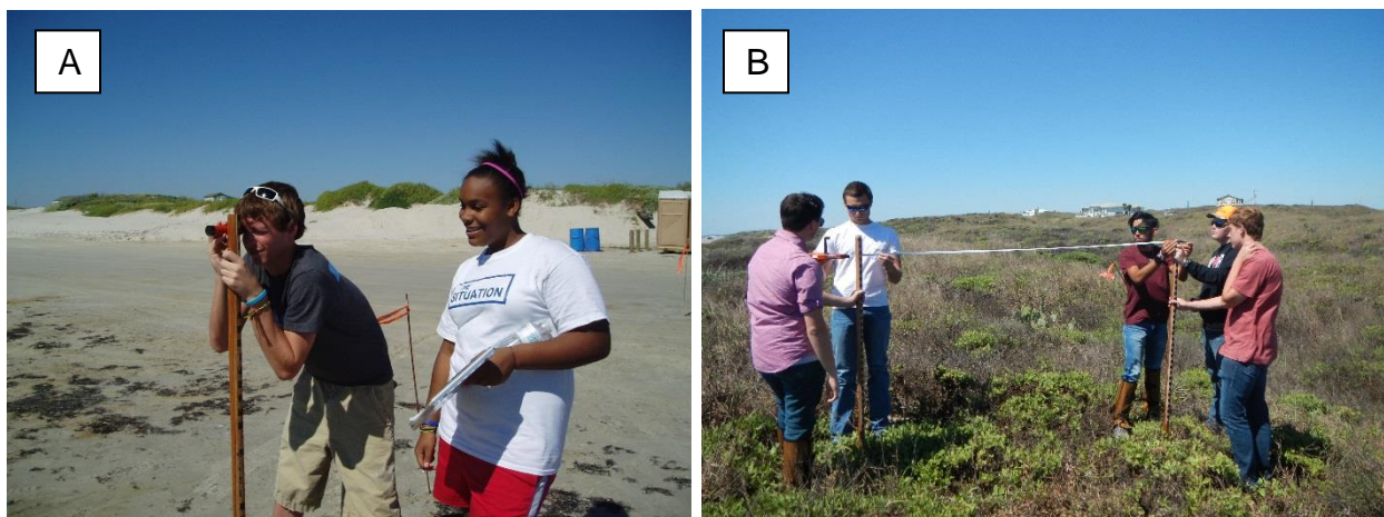
Figure 5-2. Students using (A) a sighting level to determine vertical offset between Emery rods, and (B) a metric tape to measure horizontal distance.
