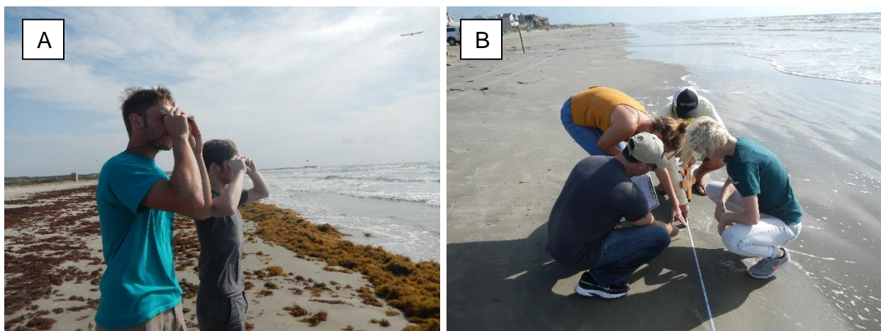
Figure 5-4. Students (A) using a sighting compass to measure wind and wave direction, and (B) measuring how far along the shoreline the float (an orange) drifted to determine longshore current.
